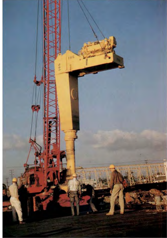
Fig. 2 - A photograph of the drilling barge CUSS I (upper left) and one of the four propulsion systems that were positioned fore and aft to port and starboard providing dynamic positioning.
